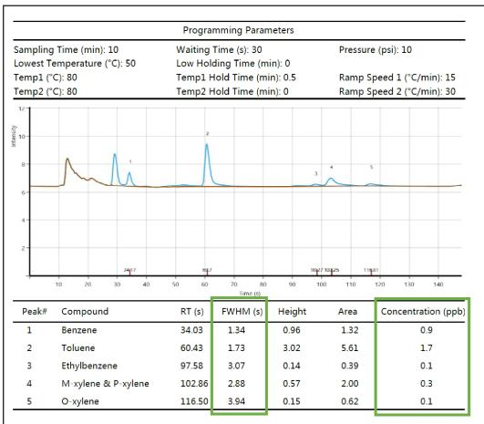
Result from a BTEX analysis in a sample vehicle using the NovaTest P100. Possible lighter/heavier compounds were not reported with the preset program of the software.
